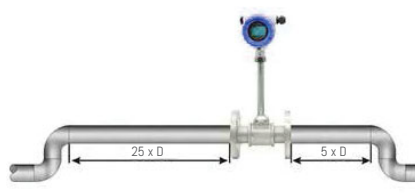
Two Square Bends At Same Plane
